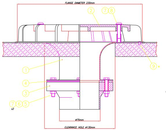
OUTLET MAY BE SUPPLIED WITH PRE-APPLIED MEMBRANE RING BONDED TO OUTLET FLANGE.
