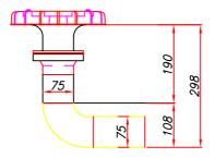
HDPE MATERIAL BUT WELDED WITH NO REDUCER.
