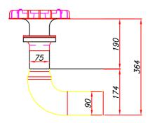
HDPE MATERIAL CUT BACK AND BUT WELDED WITH REDUCER.
